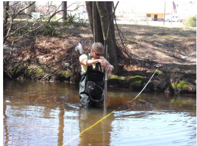
USC student measuring flow in Jackson Creek.
